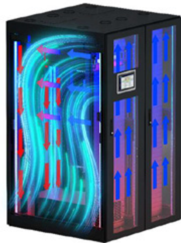
Airflow-distribution in cabinet
